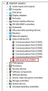
Figure 4-5: Device Manager (After Installation)
